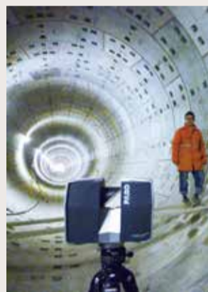
Laser scanning technology as applied in railway construction and monitoring of tunnel deformation
