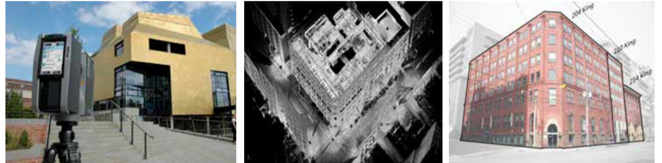
An example of a 3D building model created with PointSense Revit through post-processing of the point cloud data.
